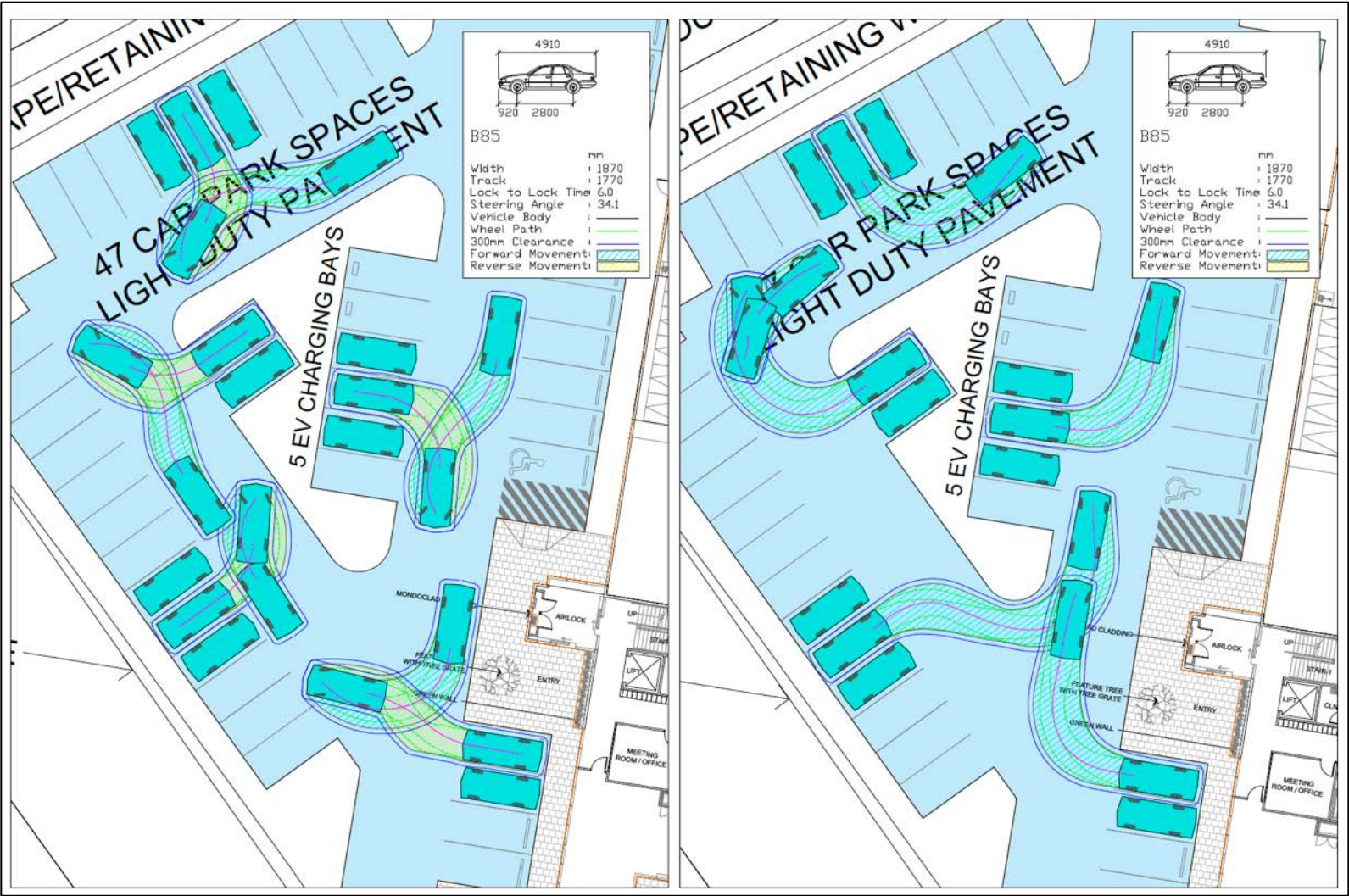
FIGURE 4.7 – 85 TH PERCENTILE VEHICLE MANOEUVRING
