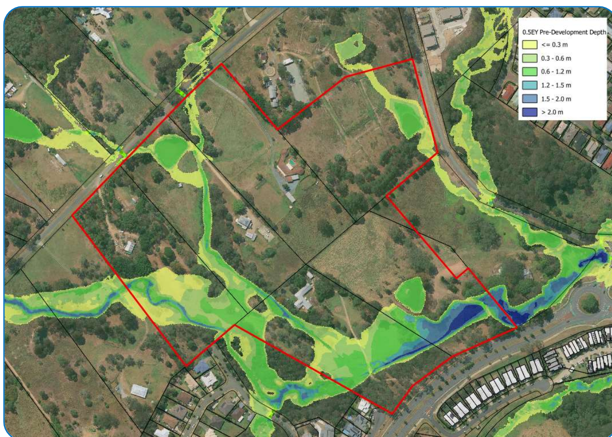
Figure 4.3 0.5EY Existing Flood Depth
