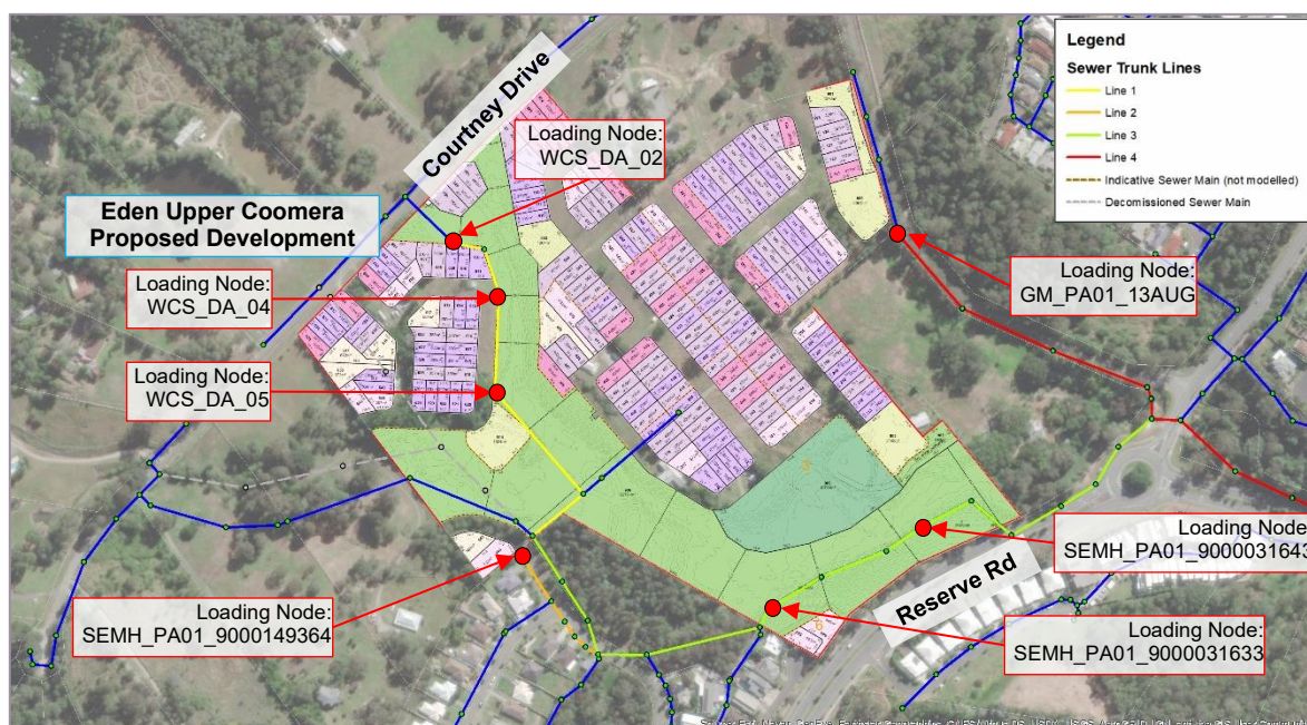
Figure 10: Wastewater infrastructure from the proposed development through to SPS PA01
