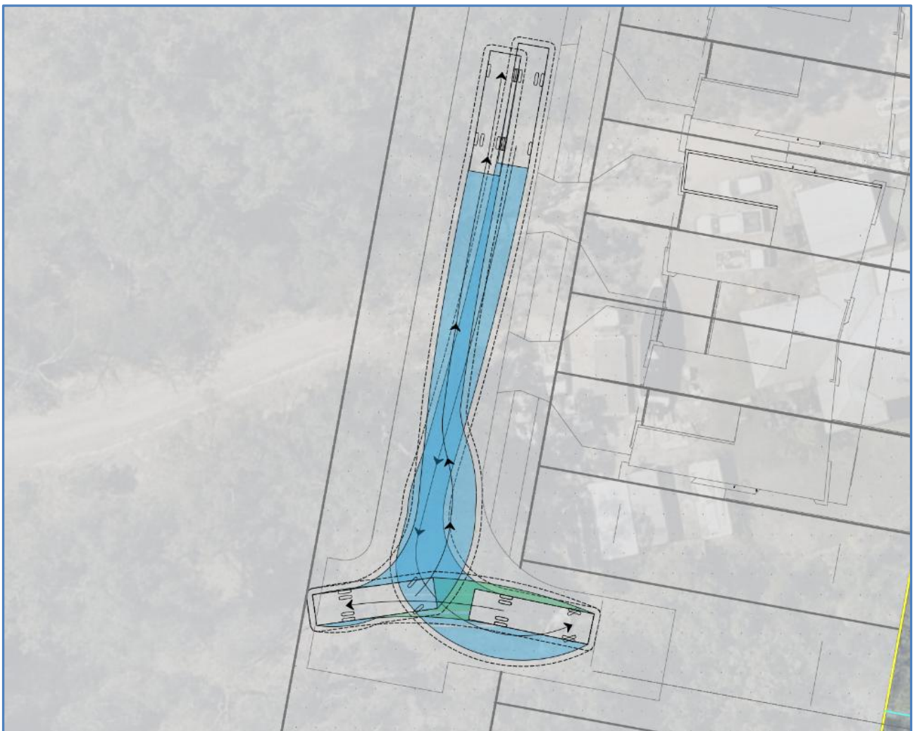
Figure 2.13: Side Loader RCV Swept Path Source: TTMC Traffic Report
