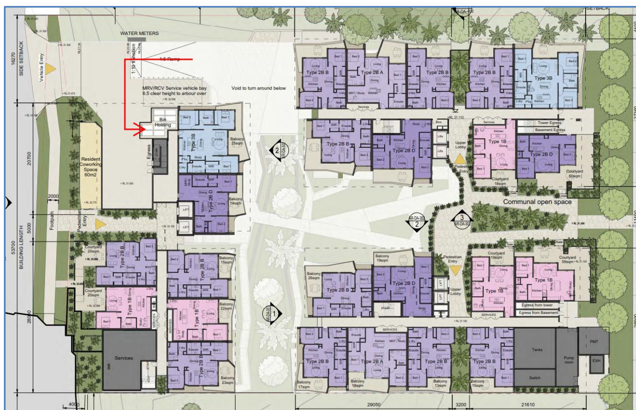
Figure 2.9: Refuse Transfer (Buildings 1 – 3)
