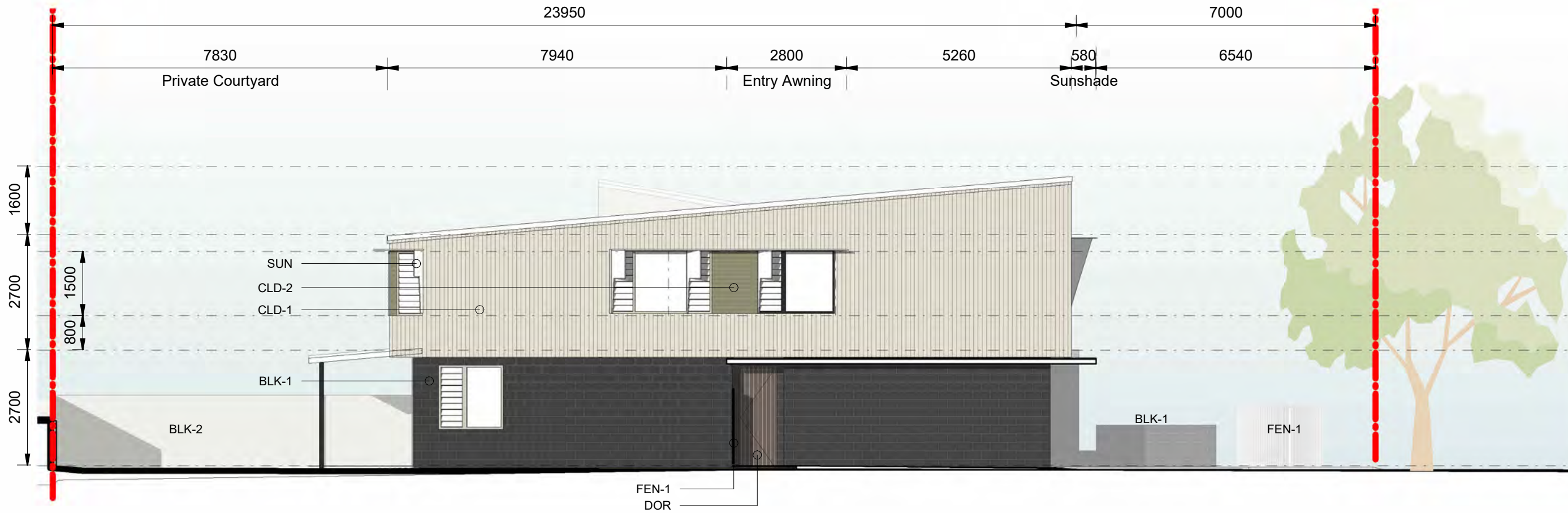
4 Townhouse Building 2 & 3 Typical North Elevation
