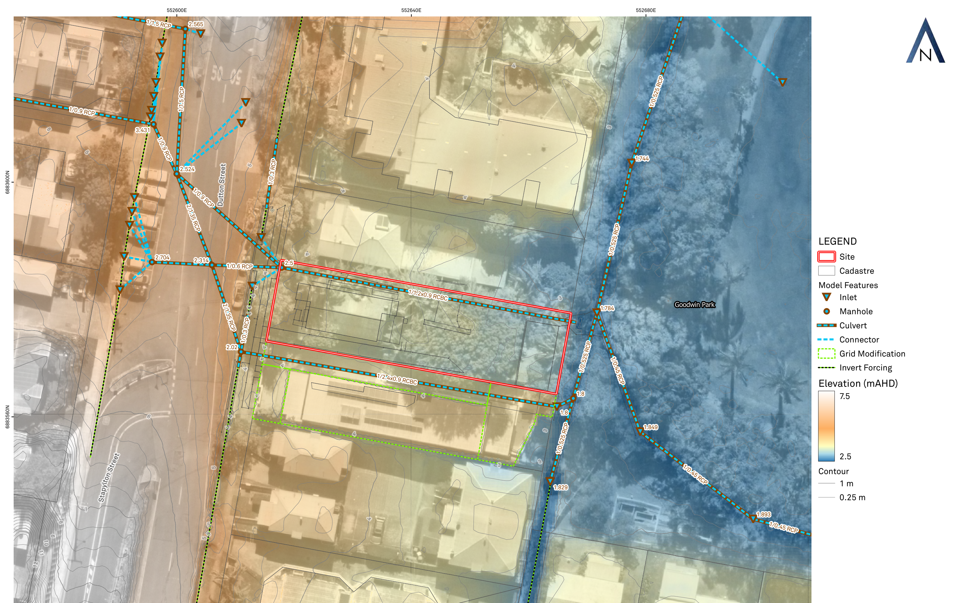
FIGURE C4 EXISTING SITE LAYOUT 60 Dutton St, Coolangatta Overland Flow Assessment Southern Cross Property Holdings
