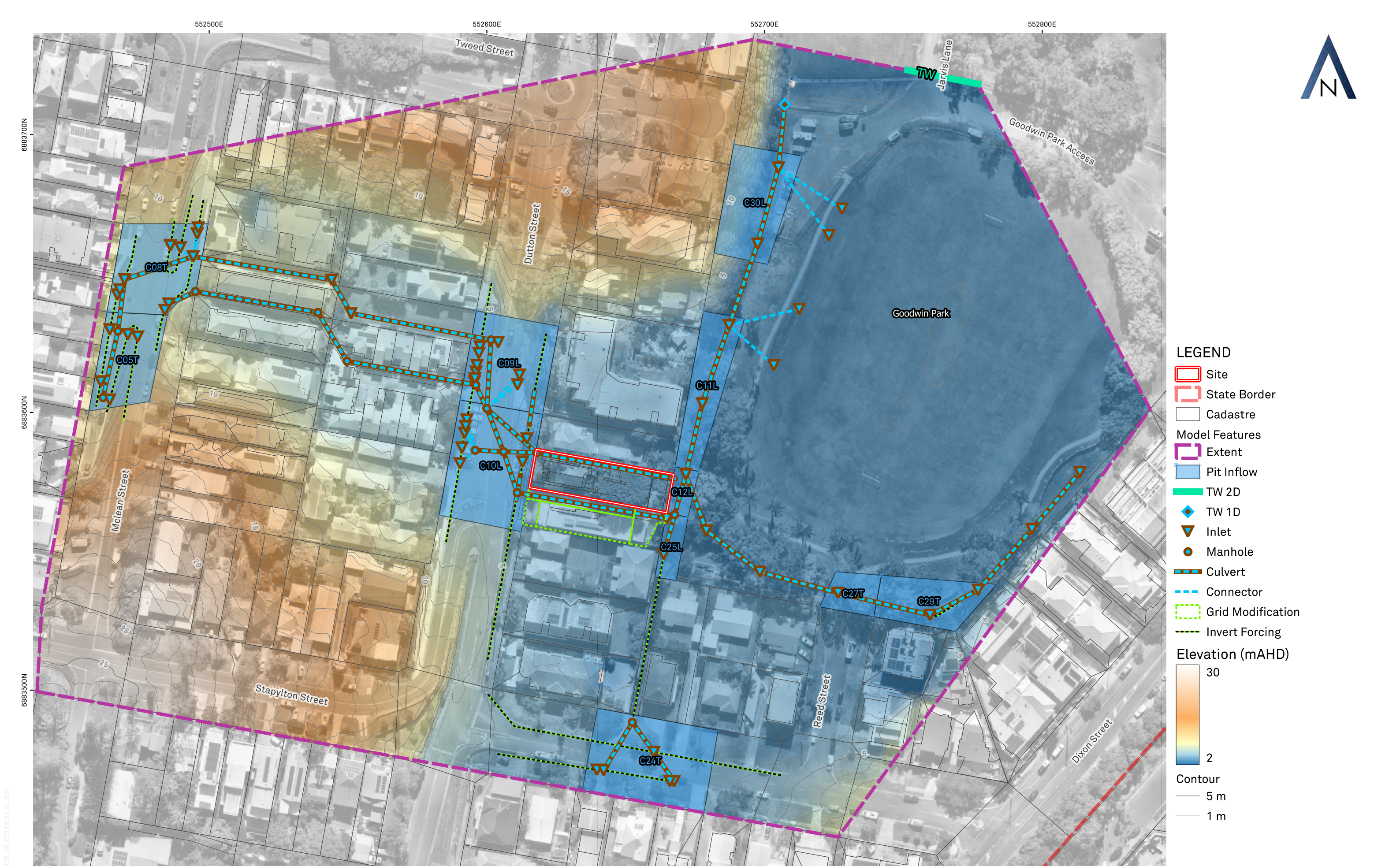
FIGURE C2 HYDRAULIC MODEL LAYOUT 60 Dutton St, Coolangatta Overland Flow Assessment Southern Cross Property Holdings
