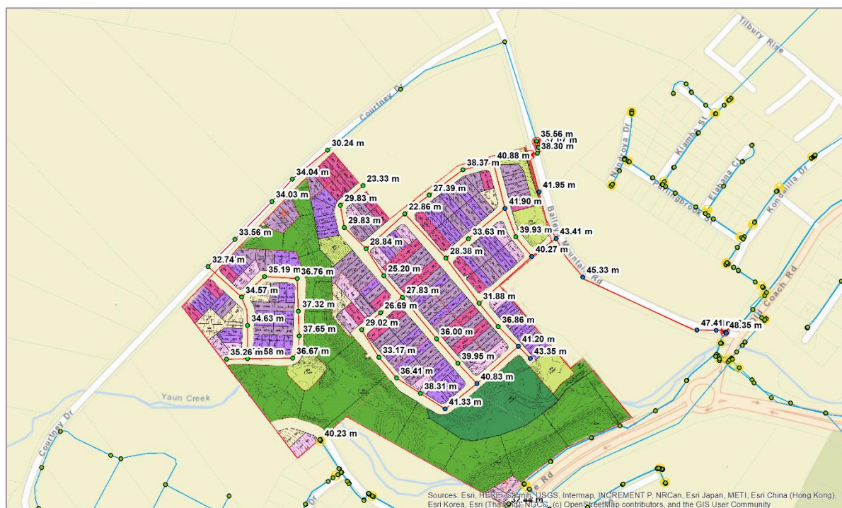
Figure 9: Peak hour internal network peak hour minimum pressure under ultimate (2066) planning horizon.
