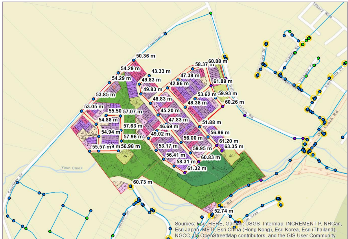
Figure 14: Peak hour internal network peak hour minimum pressure under existing (2066) planning horizon (rezoned).
