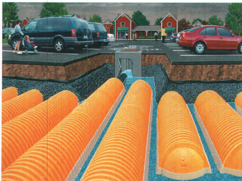
StormTech Detention System
