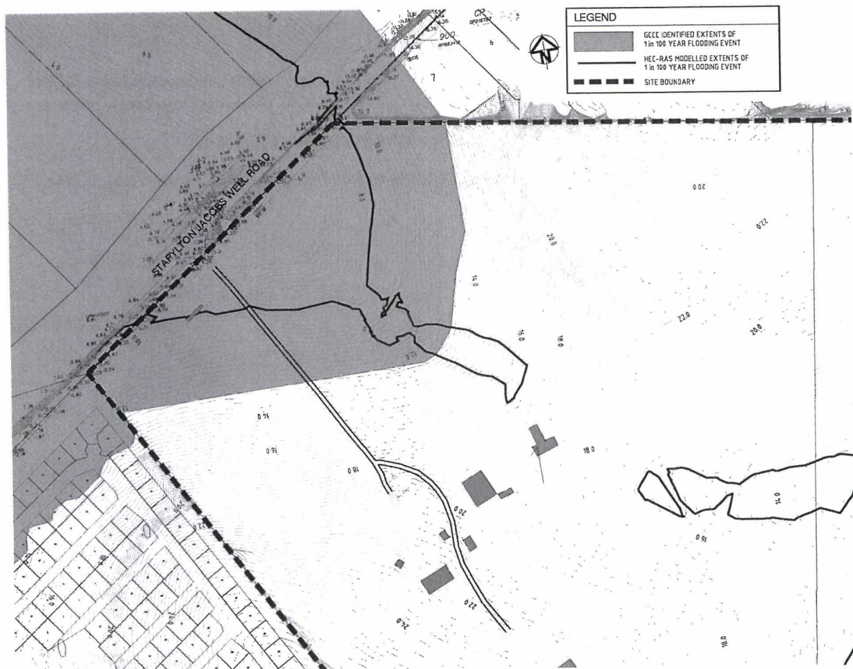
Figure 4.2 – GCCC Mapping & HEC-RAS Modelled Q100 Flooding in Plan (Local & Regional)
