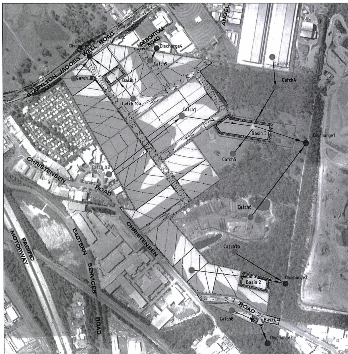
Figure 3.10 – Diagram of Developed Case XP-RAFTS Modelling Environment
