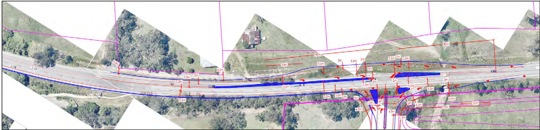
FIGURE 5.4 – SIGHT DISTANCE AT PROPOSED ACCESS POINT
