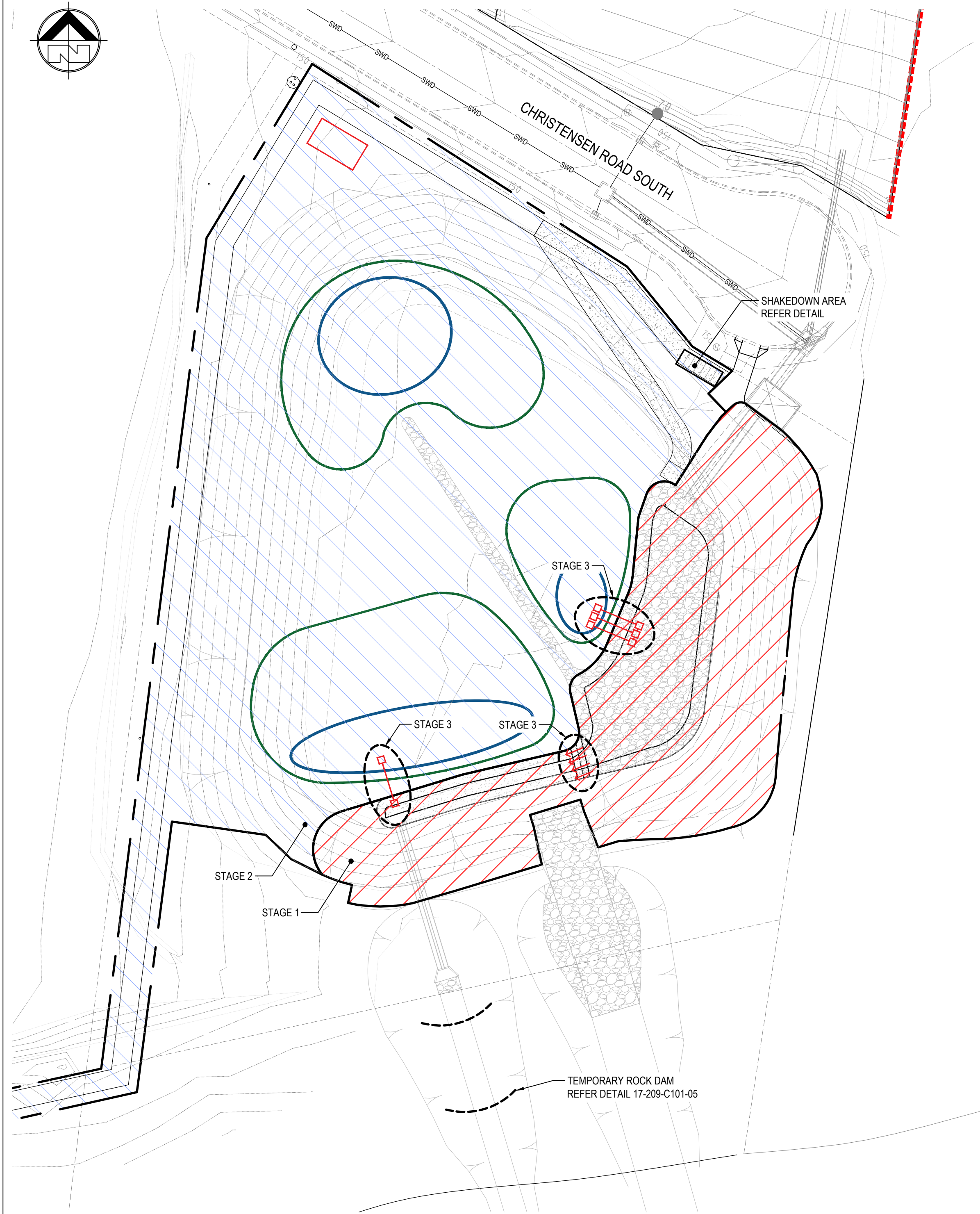
WETLANDS EROSION & SEDIMENT CONTROL PLAN SCALE 1:500 (A1)
