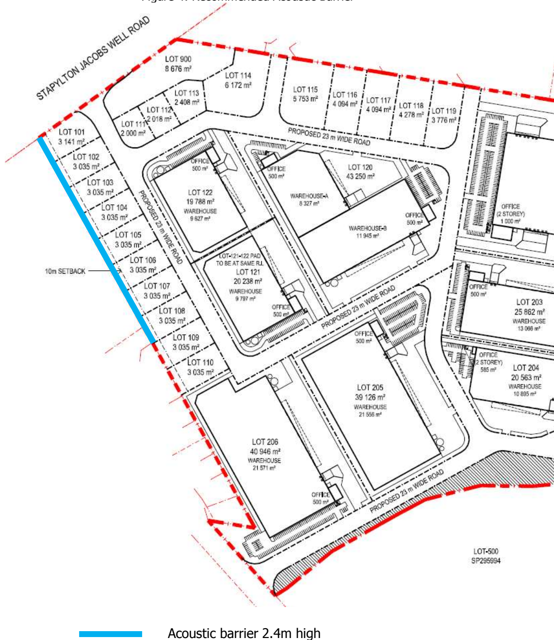
Figure 4: Recommended Acoustic Barrier
