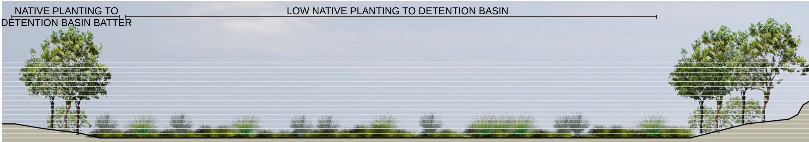
INDICATIVE DETENTION BASIN PROFILE (C-C)
