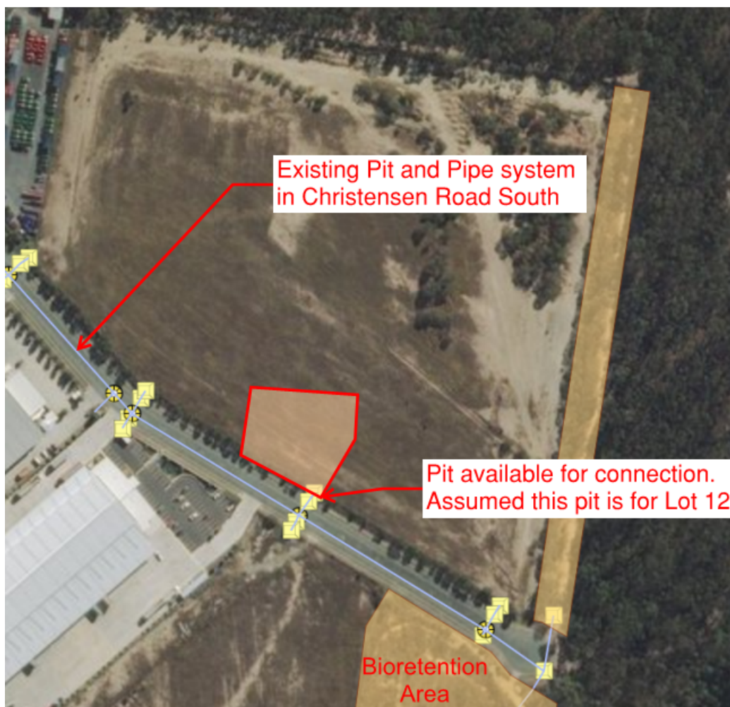
Figure 2-2 Stormwater Infrastructure (obtained 28.09.17 – COG ArcGIS)
