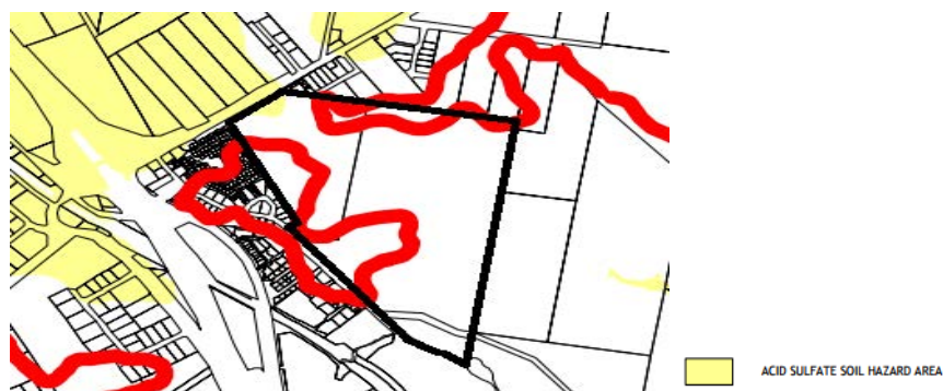
Figure 14 - Acid Sulphate Soil Hazard Areas Overlay Mapping (OM14-1) (Council mapping, 2003)
