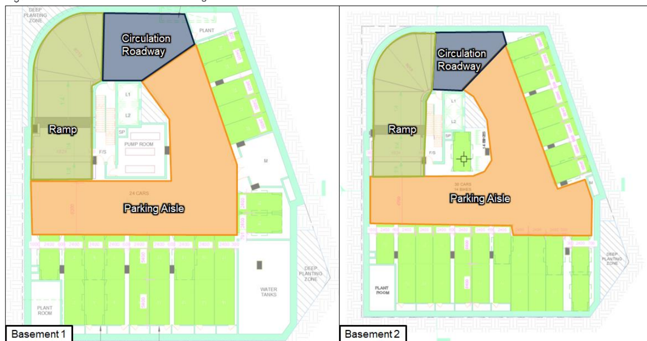
Figure 1-2 Basement Level Parking Classifications
