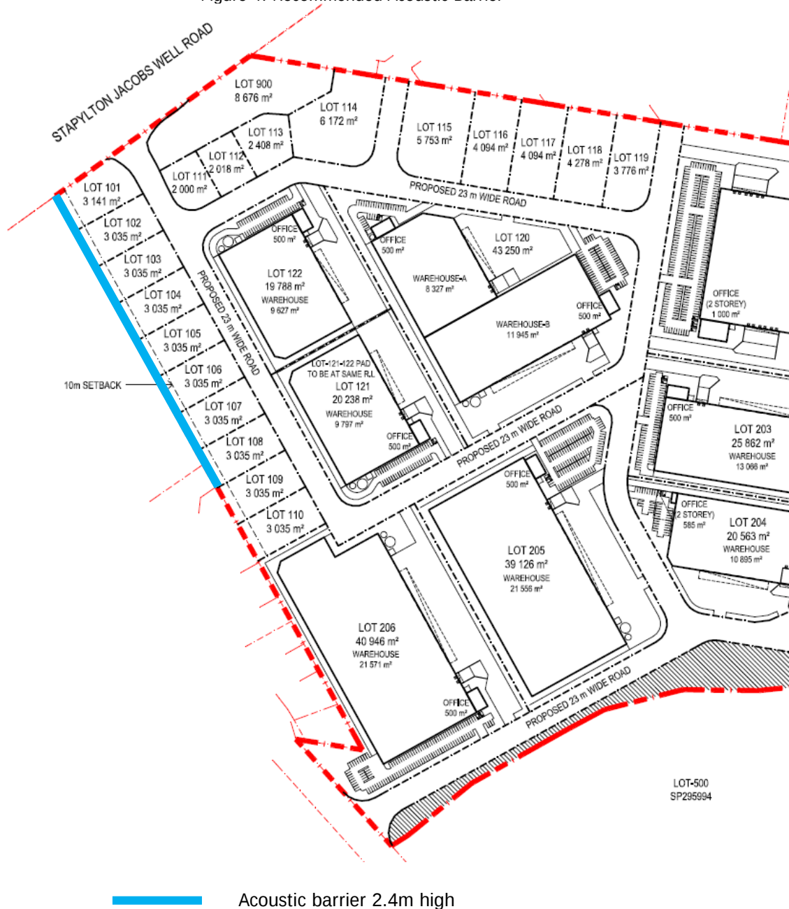
Figure 4: Recommended Acoustic Barrier
