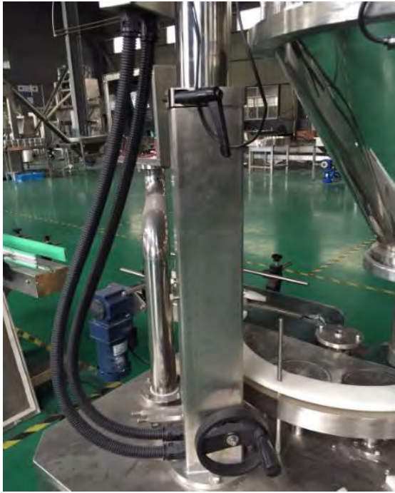
Handwheel adjust auger filler height to meet different container height need
