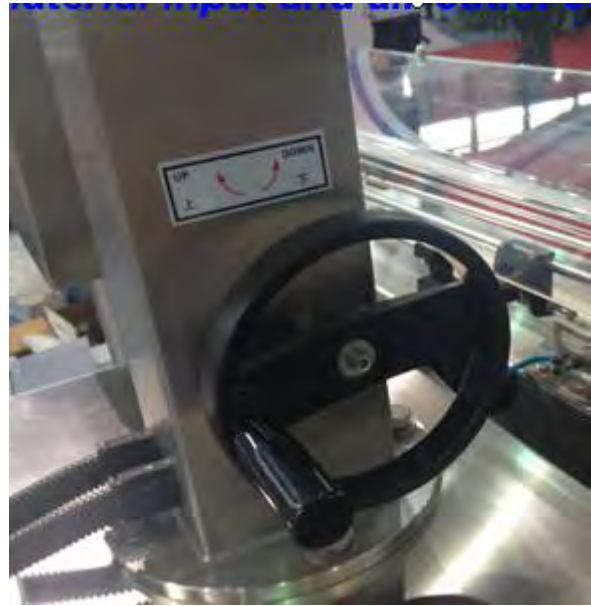
Handwheel adjust auger filler height to meet different container height need
