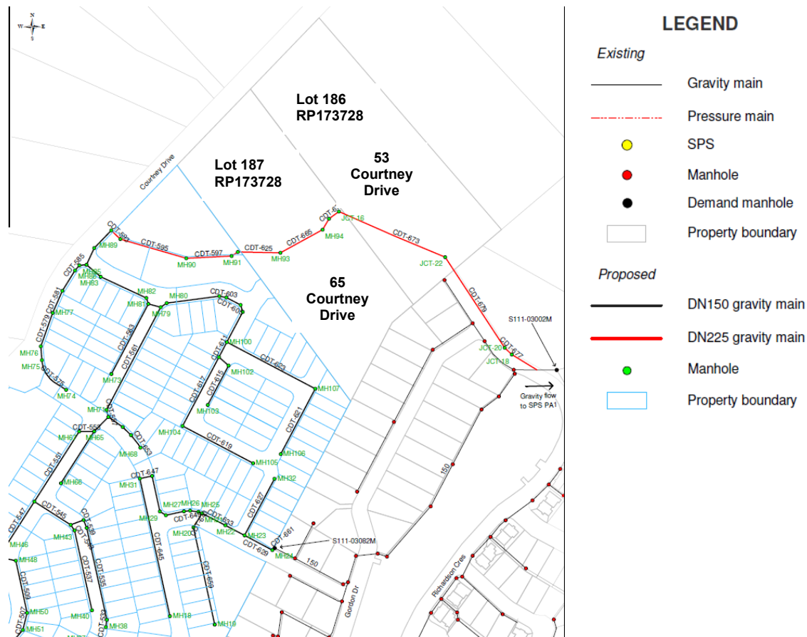
Figure 21 - Sewer hydraulic model pipe layout (Source:H2One)
